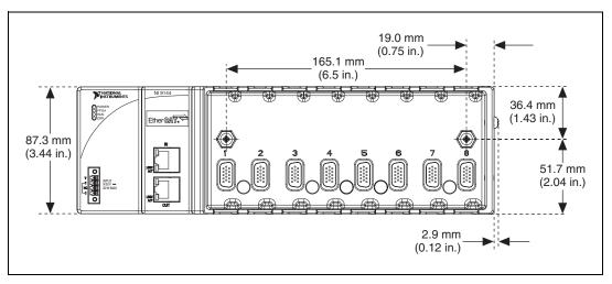
Figure 3. NI 9144 Chassis, Front View with Dimensions
